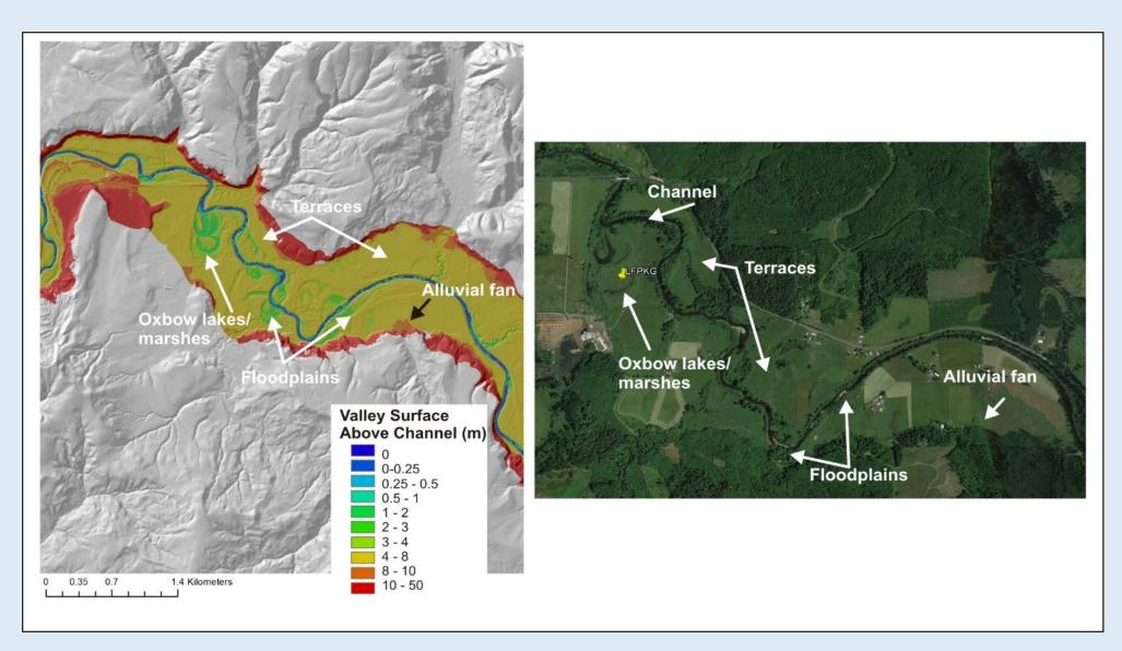
An example of two different types of valley floor and floodplain mapping in the Simonette River basin, Alberta (using 1 m LiDAR).
