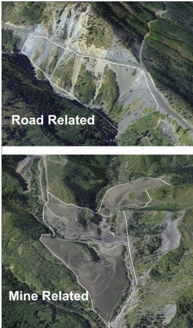
Figure 29. Controllable sources of sediment in the Coal Basin include eroding hillslopes below and above roads (upper panel) and mine related ground disturbance (lower panel). Controllable sources of sediment in Coal Basin make up approximately 2% of all potential sediment sources.
