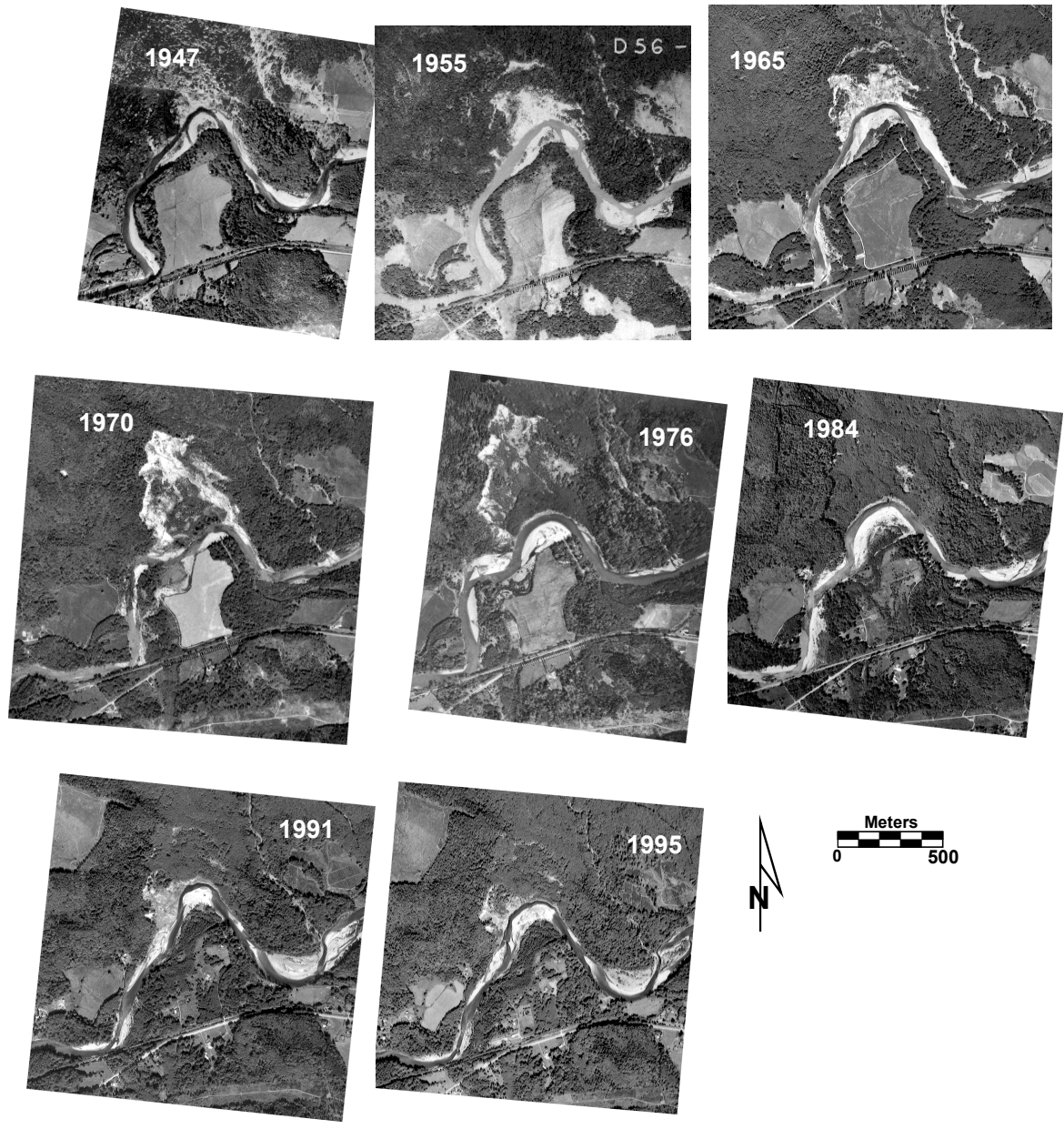
Figure 2. Aerial photograph record for Hazel landslide. Major events occurred in 1951, 1967, and 1988.
